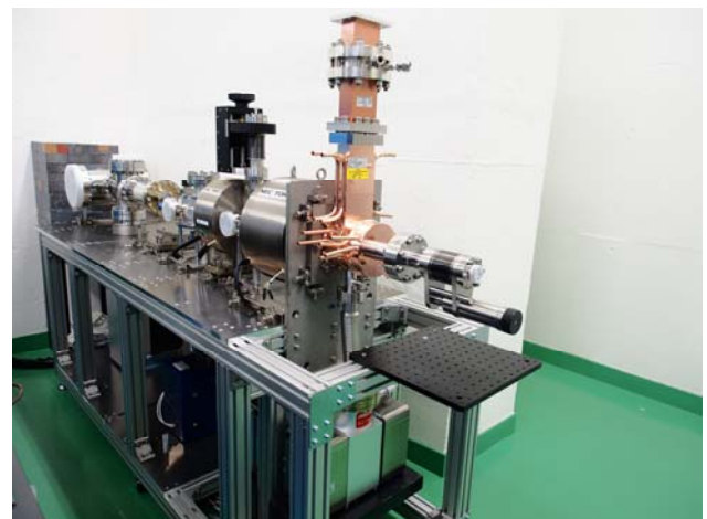
Figure 5: RF gun test facility for short-pulse and low-emittance electron beam generation.
