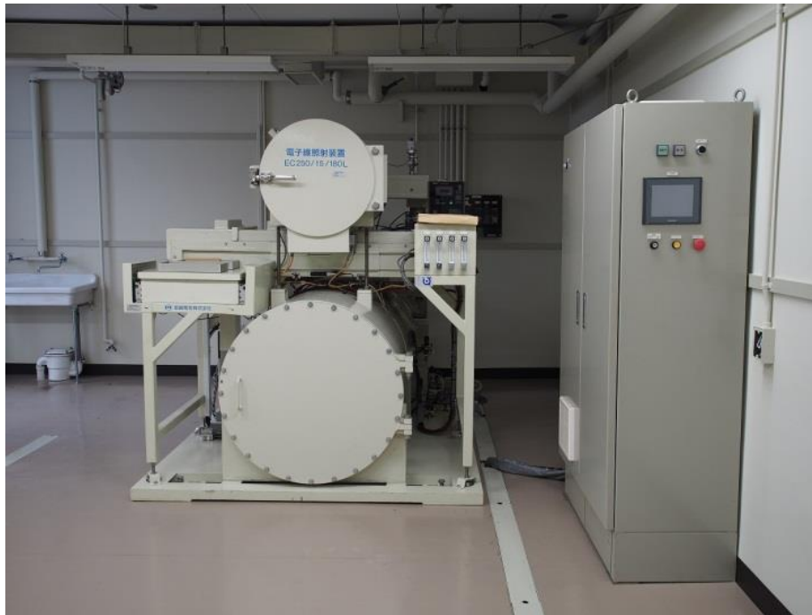
Fig.2 Relocated low energy electron accelerator (250 kV) made by Iwasaki
