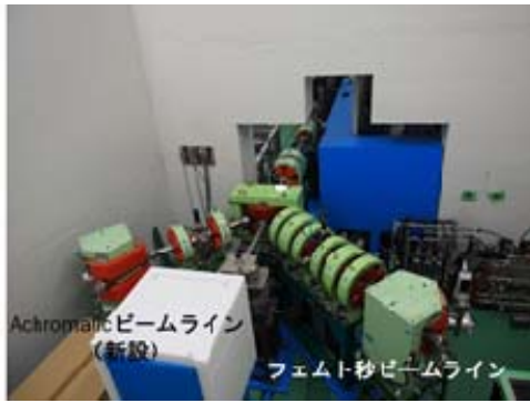
Figure 2: New femtosecond electron linear accelerator using RF gun.
