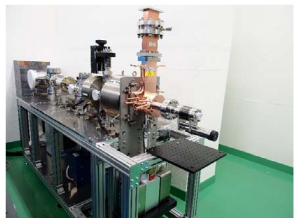
Figure 5: RF gun test facility for short-pulse and low-emittance
