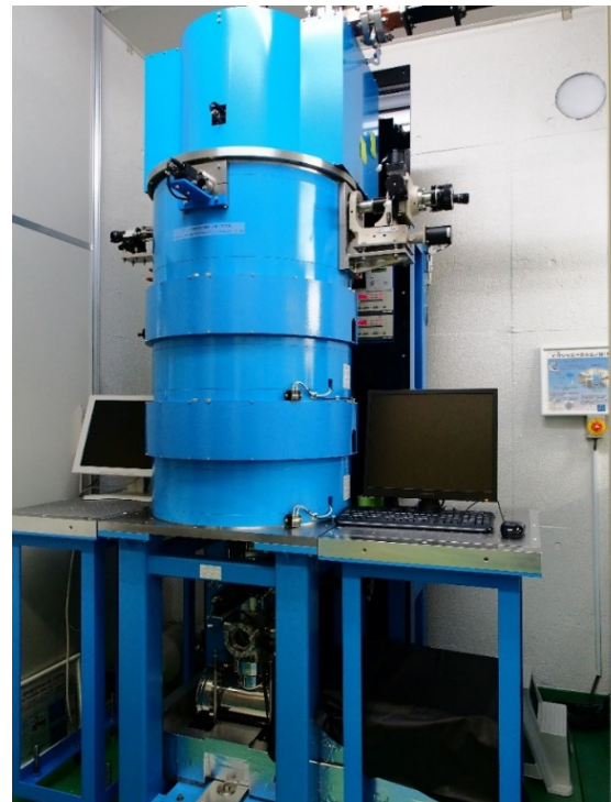
Fig. 1: The prototype of RF gun based relativistic-energy electron microscopy which was constructed at Osaka University in 2012 and improved in 2014.
