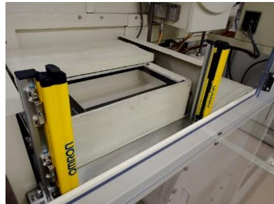
Fig.3 Curtain-like sensor for finger pinch prevention at the sample entrance of accelerator
