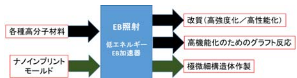
Fig.1 Functionalization of various polymer materials by irradiating of low energy electron beam
