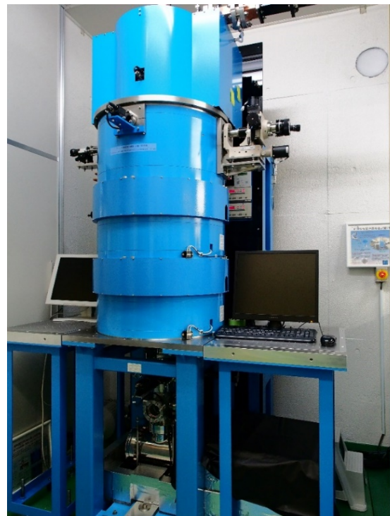
Fig. 1: The prototype of RF gun based relativistic-energy electron microscopy which was constructed at Osaka University in 2012 and improved in 2014.
