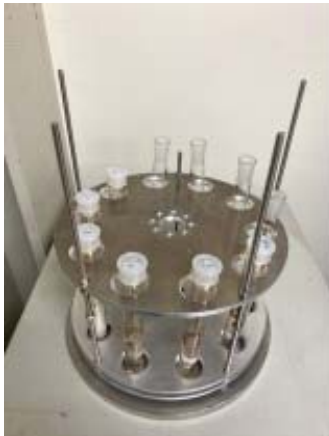
Fig.1 Sample holder for \gamma -rays irradiation
