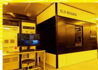
State-of art ultra-fine electron beam lithography system
