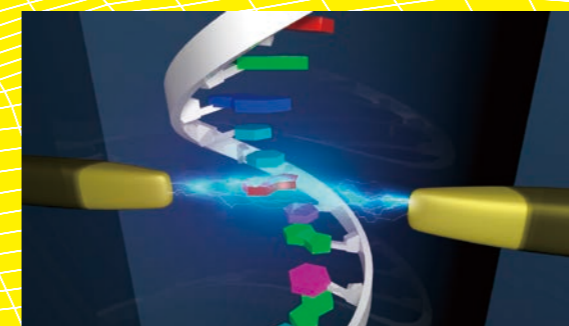
Figure: Operating principle of single-molecule quantum sequencing to determine base sequences and identify chemically modified base molecules. ©Takahito Ohshiro et al.
