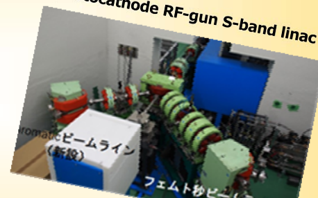
New femtosecond electron linear accelerator using RF gun.
