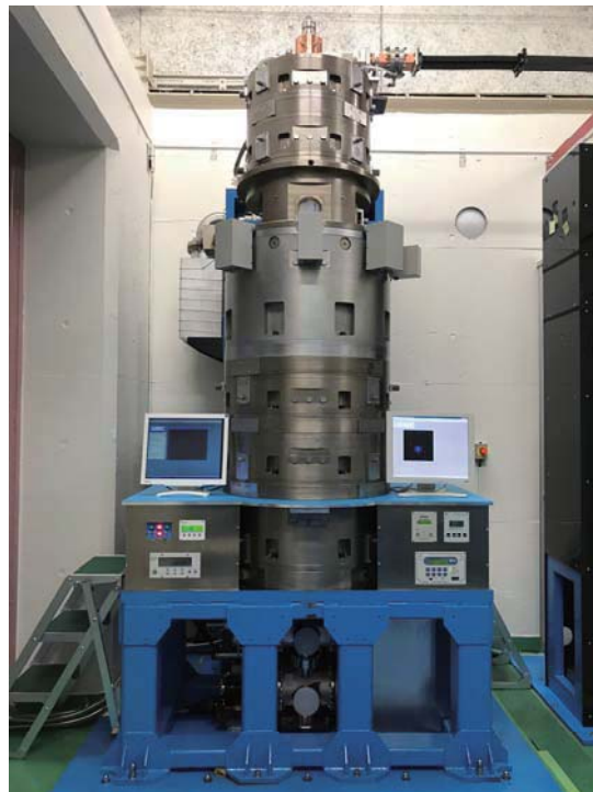
Figure 1: Ultrafast electron microscopy using relativistic-energy femtosecond electron pulses.
