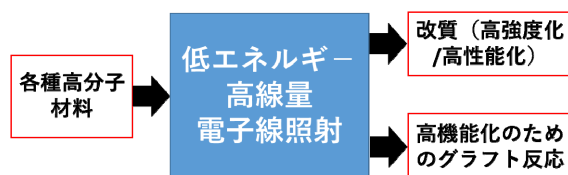
Fig.1 Functionalization of polymer materials by low energy and high dose electron beam
