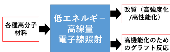
Fig.1 Functionalization of polymer materials by low energy and high dose electron beam
