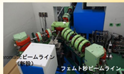
New femtosecond electron linear accelerator using RF gun.
